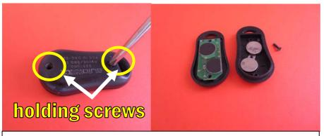
Unscrew 2 small screws at the back of plastic shell. Open remote and separate in 2 parts: **part 1**- top hard shell with button key pad and electronic board and **part 2**- hard shell with two batteries.
