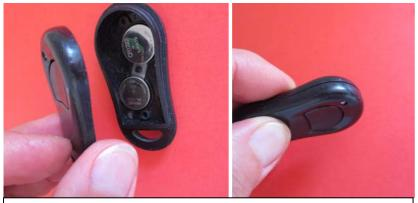
Next place part with mounted electronic board over bottom part of shell. If all components are correctly positioned you can close remote and screw it together.
