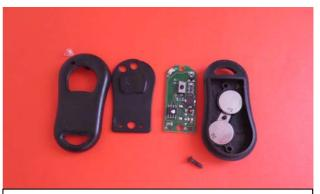
Your remote is separated and ready for insertion of new Silicone repair pad.
