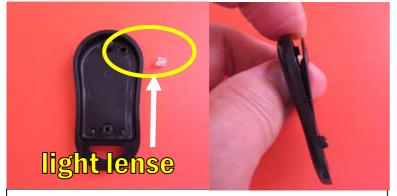
Once lense is removed you can push old key pad out from plastic shell using your thumb.
